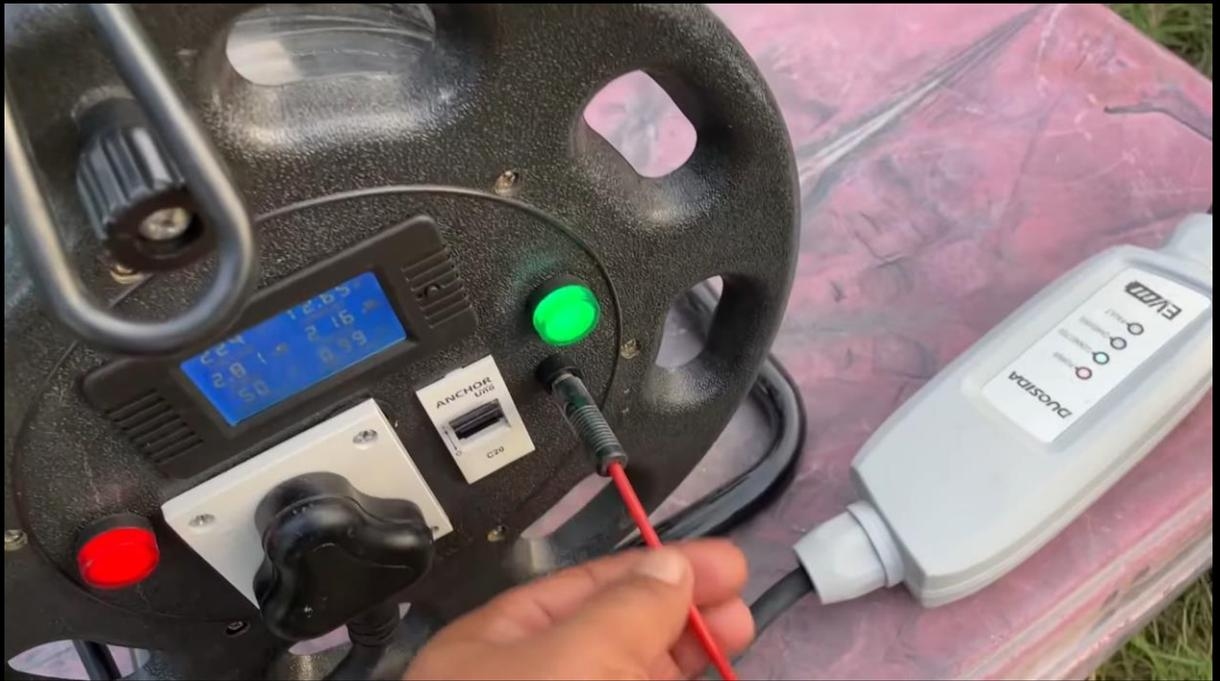
Connect the banana plug from the earthing wire to the charger.
